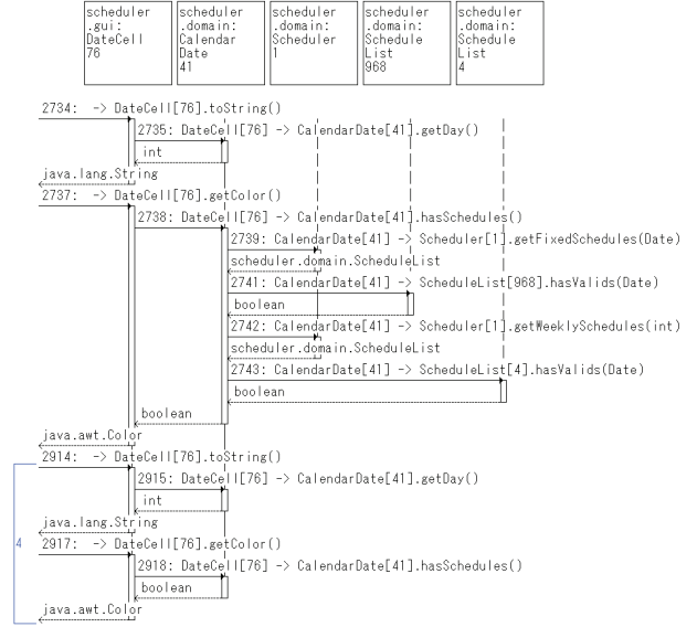
Figure 1. An extracted sequence diagram representing an interaction scenario \langle s_4, t_3 \rangle : a DateCell requests schedule data to a CalendarDate.
